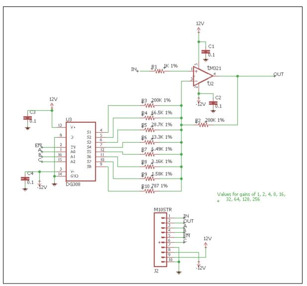
Figure 11-4 Variable Gain Module
