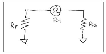
Figure 4-1 Measurement Using a Simple Ohm Meter
