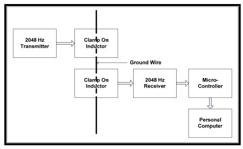
Figure 7-1 Simplified Ground Ohms System Block Diagram
