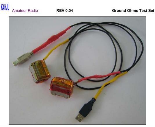
Figure 6-6 Clamp-On Inductive Transducers
