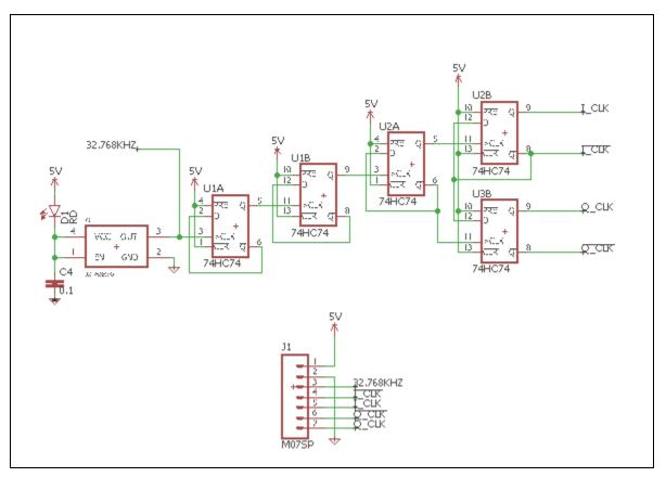
Figure 11-1 I Q Generator Module
