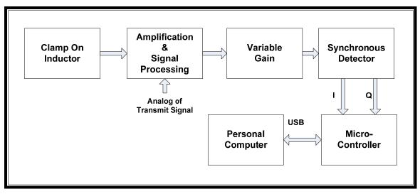
Figure 7-3 Simplified GroundOhms Receiver Block Diagram
