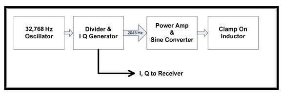
Figure 7-2 Simplified Ground Ohms Transmitter Block Diagram
