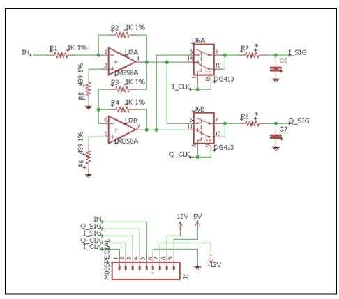
Figure 11-5 Synchronous Detector Module
