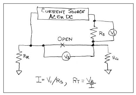
Figure 4-2 Measurement Using a Four Terminal Measurement System
