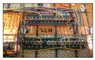
Figure 5-2 Insulation Displacement Wiring
