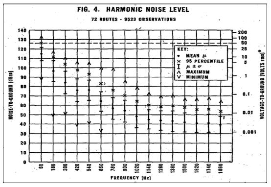
Figure 7-4 Typical Power Line Induced Noise On Telephone Cable
