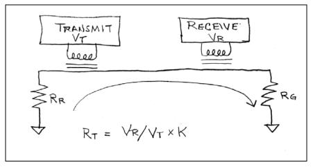
Figure 4-3 Measurement Using Inductive Coupling
