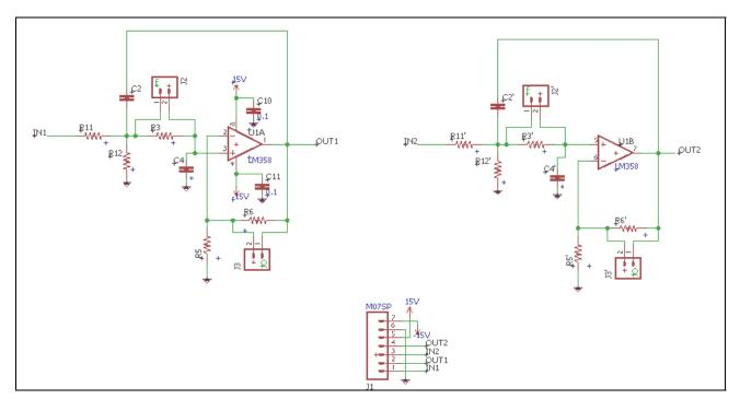
Figure 11-6 Low Pass Filter Module
