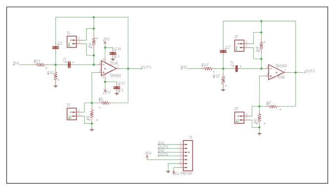
Figure 11-3 Band Pass Filter Module
